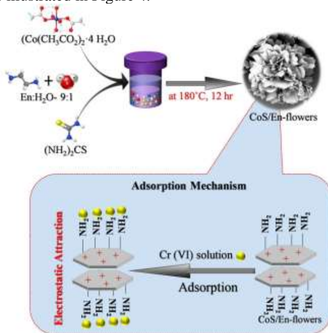
Figure 4 Schematic illustration of processing steps of CoS/En-flowers adsorbent and mechanism of Cr(VI) ions adsorption on amine functionalized CoS surface
